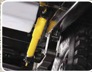
For smoother trips, Baja camping trailers are built with leaf springs and shock absorbers.
